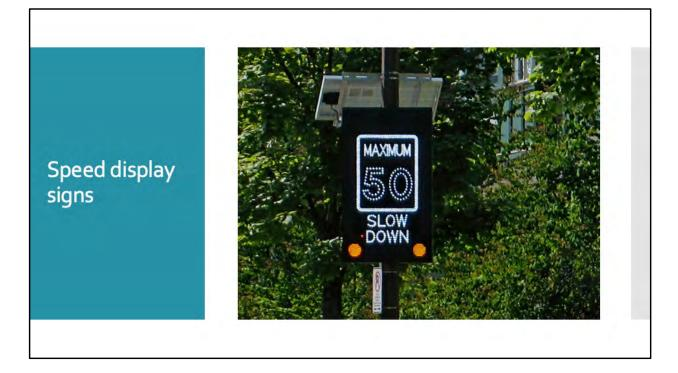
Sign incorporates a radar speed detector and is activated by a vehicle travelling above a pre-determined speed threshold Reduces 85th percentile traffic speeds of approximately 10 km/h (example from UBC)
